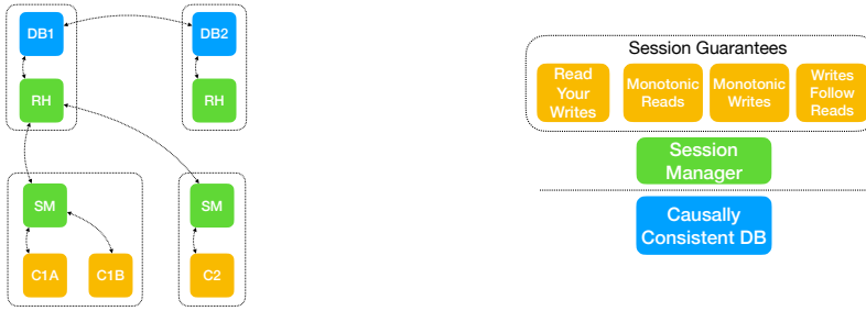
Fig. 9. Clients using the distributed database via the session manager library. Fig. 10. Vertical compositionality of specifications.
